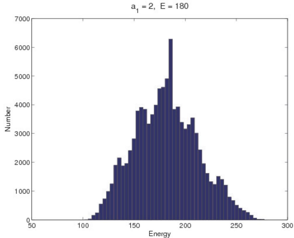
**The sawtooth modulated quartic oscillator: The histogram (distribution) of the final energies of the microcanonical ensemble after 100 iterations (periods of length  $2T$ ).**
