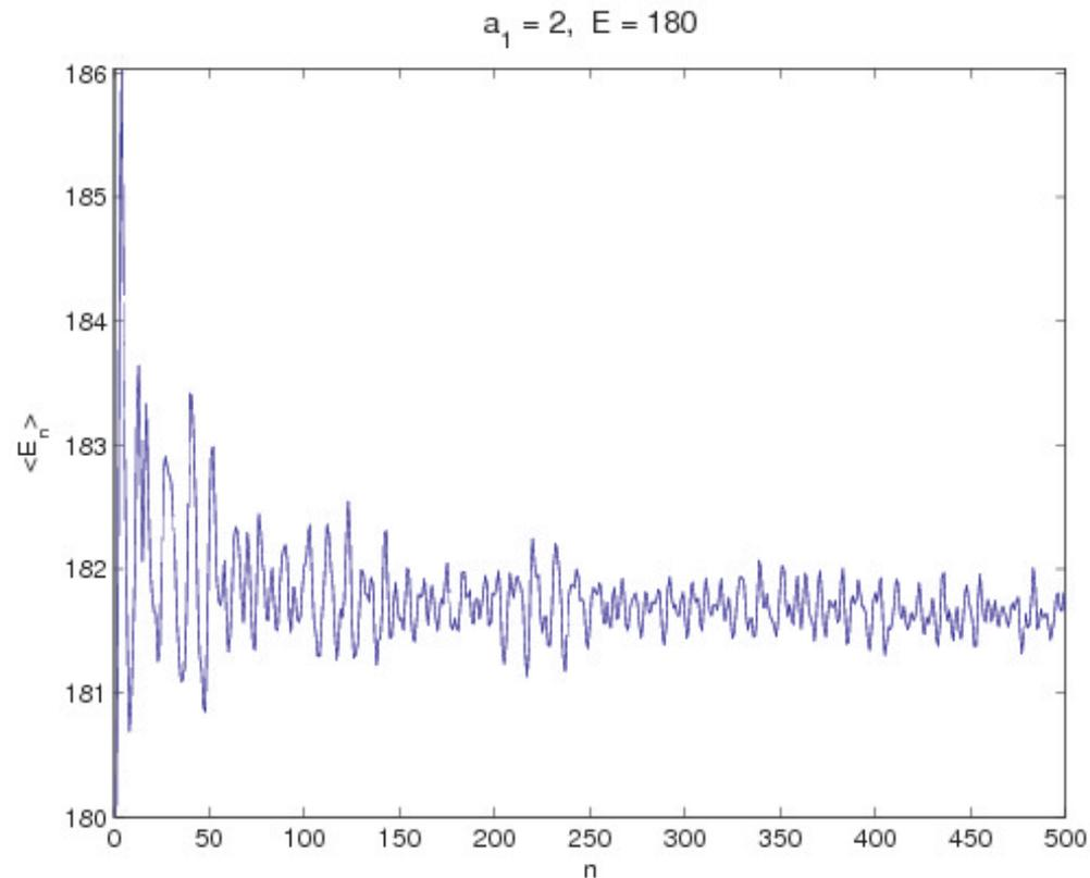
**The sawtooth modulated quartic oscillator: The average energy of the initial microcanonical ensemble as a function of the number of iterations  $n$ , for 1000 initial conditions.**
