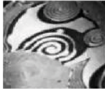
Fig. 21. Spirals during single crystal catalysis of CO-oxidation on Pt(110) [44].
