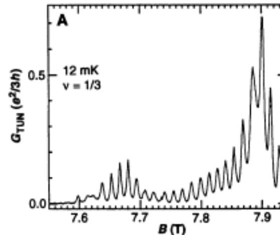
**The Aharonov-Bohm effect gives fluctuating current across the quantum dot - the period determines the charge to  $e/3$  !**
