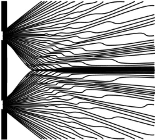
**Fig. 2** Bohmian trajectories in a double-slit experiment [15]. The key parameters used in [15] follow that in Jönsson's experiment [28]: slit half-width  $a/2 = 0.1 \times 10^{-4}$  cm, slit separation  $d = 1 \times 10^{-4}$  cm, distance between the slits and the screen  $x = 35$  cm, and the electron de Broglie wavelength  $\lambda = 5.5 \times 10^{-10}$  cm.
